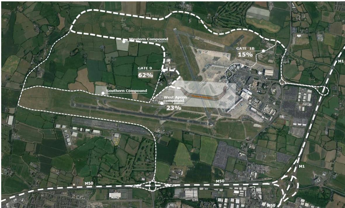
Figure 13 Site Access & Haul Routes Phase 2 (During closure of Runway 16/34)
